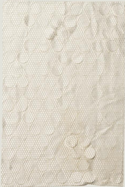
Technique: Lasercutting (power 50 % speed 100 %) Material: High Visibility Jacket lining, 100 % polyester Source: Workwear collected by VAER
