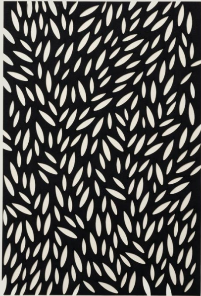
Technique: Lasercutting (75 % power, 40 % speed) Material: Faux Suede Waterborn*, 85% polyester 15% polyurethane Source: KVADRAT
