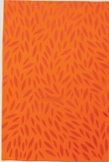
Technique: Silk screen printing with reactive colours (Printperfekt Lac Flex binder) Material: High Visibility Jacket, 100% polyester Source: Workwear collected by VAER
