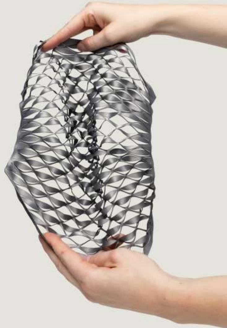
Technique: Lasercutting (75 % power, 40 % speed) Material: Black out curtain Nightfall (1308), 100% polyester FR, 32% polyester Source: EVADEK1
