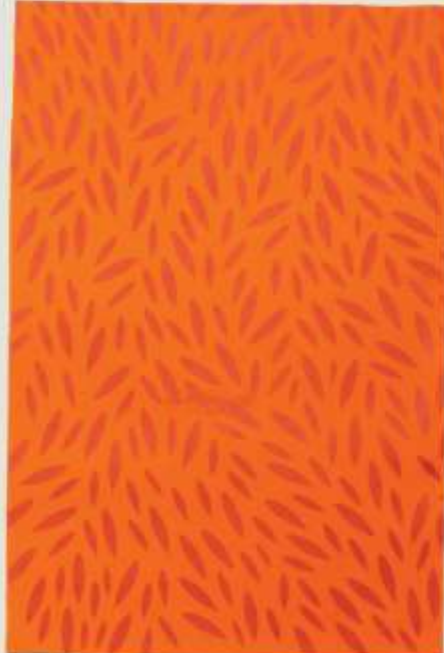
Technique: Silk screen printing with reactive colours (Printperfect Lac Flex binder) Material: High Visibility jacket, 100% polyester Source: Workwear collected by VAEI
