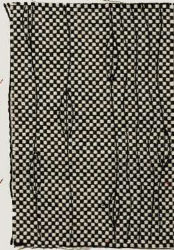
Technique: Machine Embroidery (jute stitch) Material: Upholstery Silu (8088), colour 185, 81% new Norwegian wool 19% new New Zealand wool 1% nylon Source: KVADRAT
