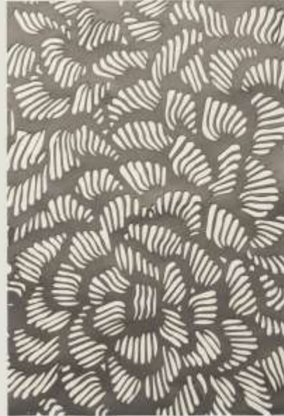
Technique: Lasercutting (75 % power, 40 % speed) Material: Black out curtain Nightfall (1308), 100% polyester FR, 32% polyester Source: EVADEK1
