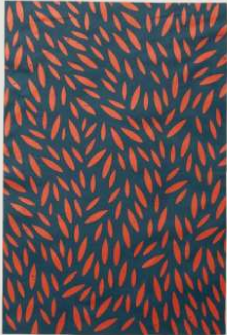
Technique: Silk screen printing with reactive colours (Printperfect Lac Flex binder) Material: Tents, polyester Source: Collected from festivals by Our Shift
