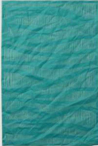
Technique: Lasercutting (power 50 % speed 100 %) Material: Tints, polyester Source: Collected from festivals by Our Shift
