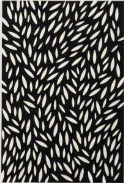
Technique: Lasercutting (75 % power, 40 % speed) Material: faux Suede Waterborn®, 85% polyester, 15% polyurethane Source: EVADEK1
