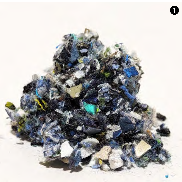
2. Batch of discontinued textile samples from Kvadrat shredded into 5 mm fibres. The discontinued textile samples are milled into varying fibre lengths all between 5 and 15 mm. This is done to research what happens with design qualities and material properties when this fluctuating waste stream is milled.
